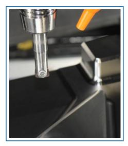
Millstar's ABL tooling system uses an innovative hybrid ball lens design to provide a large end face radius – typically equal to the diameter. This allows up to twice the step-over to greatly decrease your cycle time without sacrificing surface finish. ABL is a great option for 5 axis milling as well as 3 axis.
