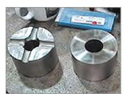
Roughing is done with a 1/2 inch (12.7 mm) Millstar carbide ball insert tool with stiff carbide shank and V-brazed tool head. The shank is held in a shrink-fit adapter. Cutting strategy is Z-level back and forth along the length of the half-round channels, inside-outside pattern, and ramp engage.
